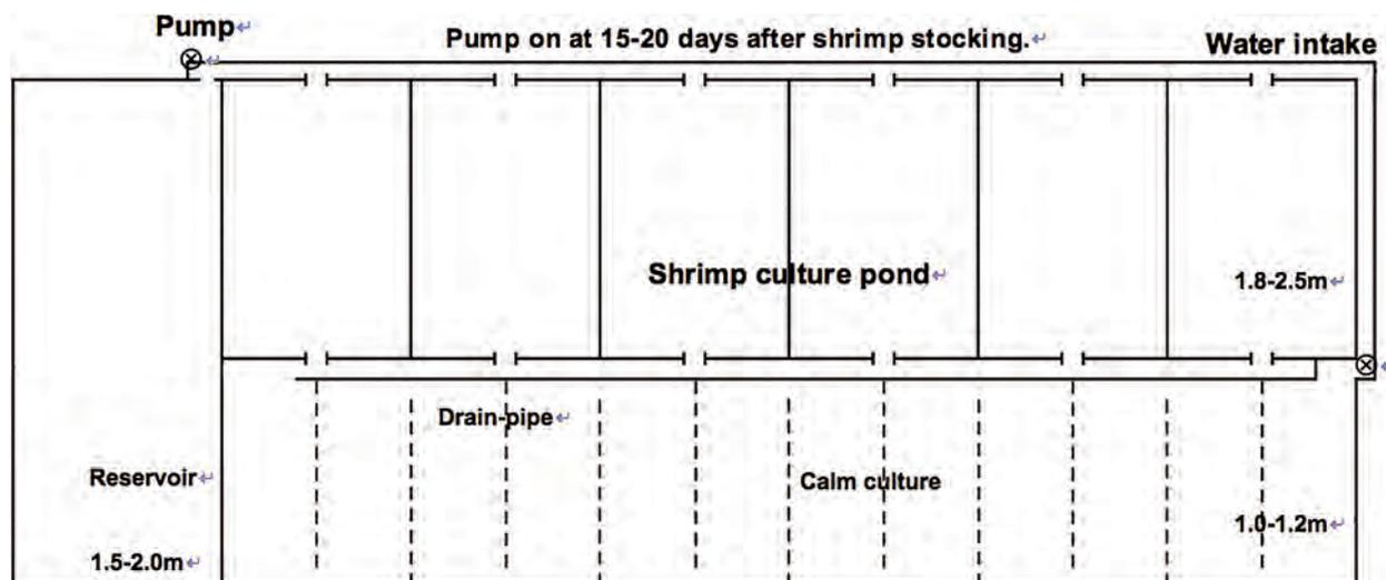
Fig. 6. Schematic diagram of the recirculating system for shrimp and clam culture in Zhejiang Province.
