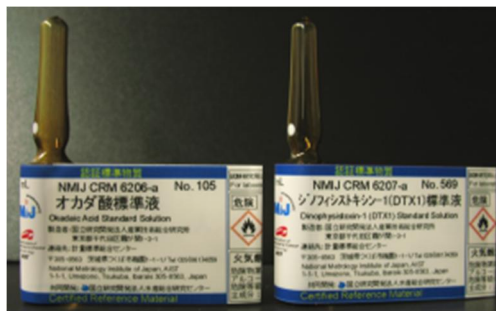
Figure 1. Certified reference materials for shellfish-poison testing Okadaic acid standard (left), Dinophysistoxin-1 standard (right) solutions
