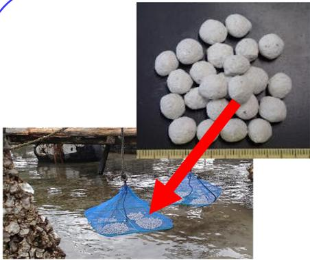
Care-shell solids made of processed oyster shells are placed in aquaculture net that has been installed in intertidal zone. Oysters will later attach to care shell.
